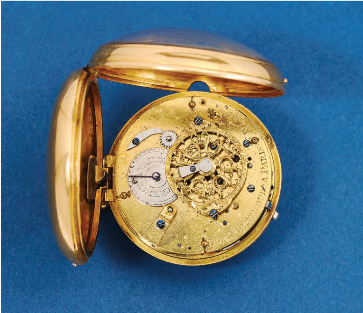
7. LOUIS (PIERRE-LOUIS) BERTHOUD, Paris, c. 1810, No. 4410, key-wind movement with verge escapement and dumb quarter-repeating, enamel dial signed Ls. Berthoud, 44mm.
