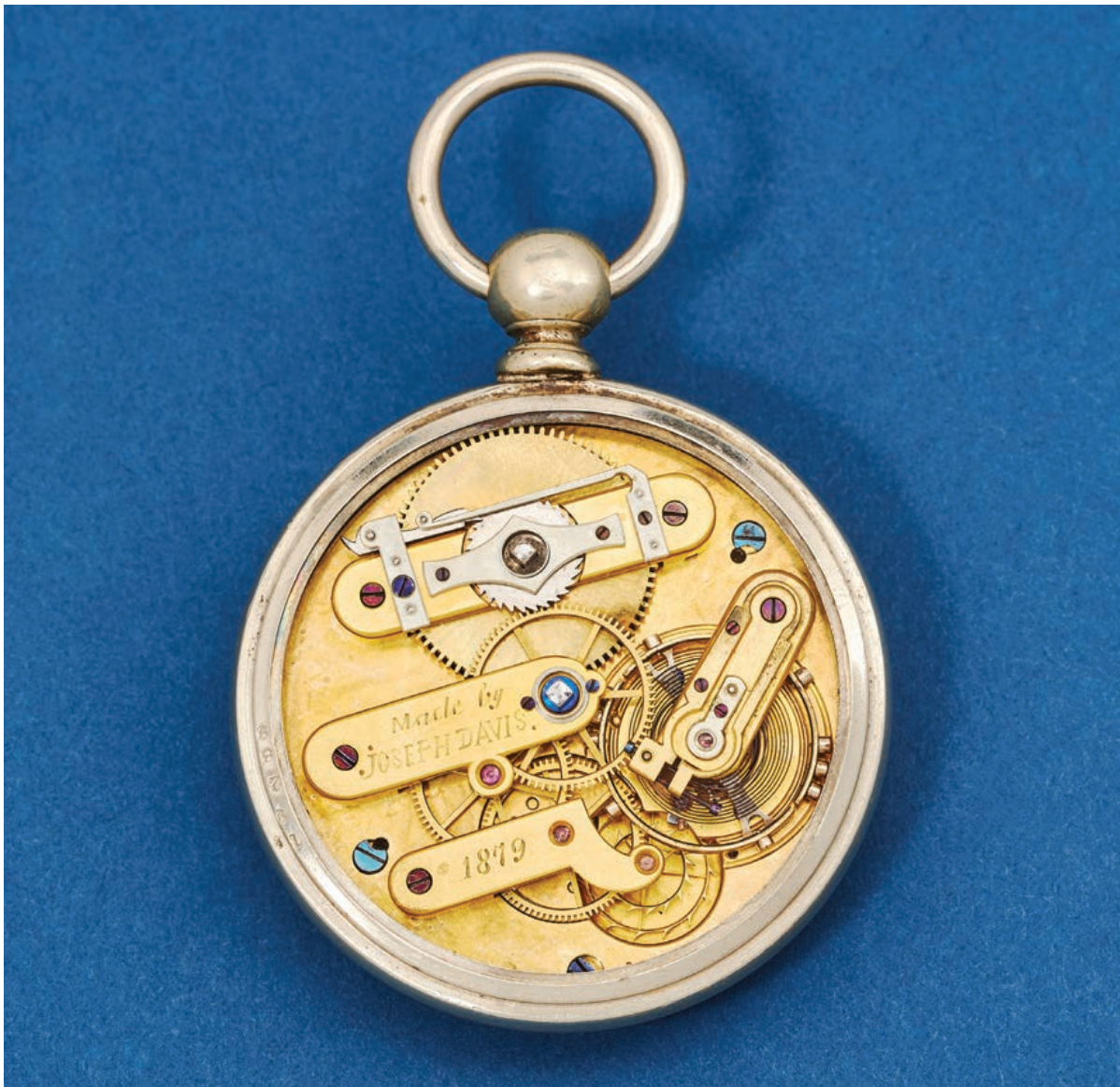
25. CHARLES FASOLDT, Albany, c. 1860, No. 114, movement engraved "Joseph Davis, 1879," later cased, key-wind 16-jewel movement with co-axial escapement invented by Fasoldt, 57mm.
