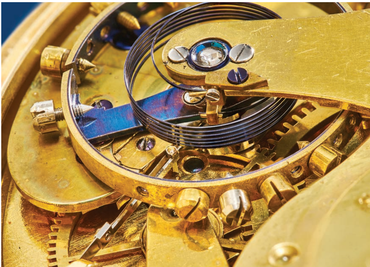
No.27, BARRAUDS & LUND, Earnshaw spring-detent escapement
